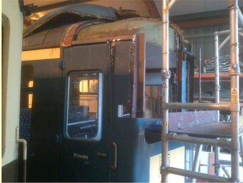
*Stripped cab of M50528 (L.Railcars)*
