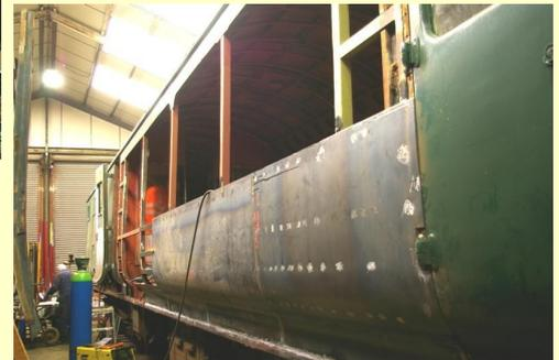
*Progression of bodywork repairs to 56097, showing new framework and metal panelling (Llangollen Railcars)*
